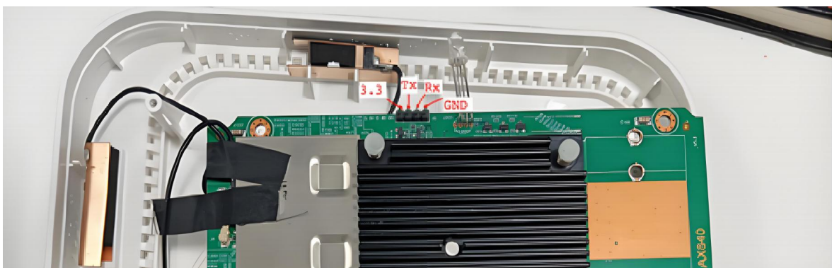
Connection between TTL and AP:
